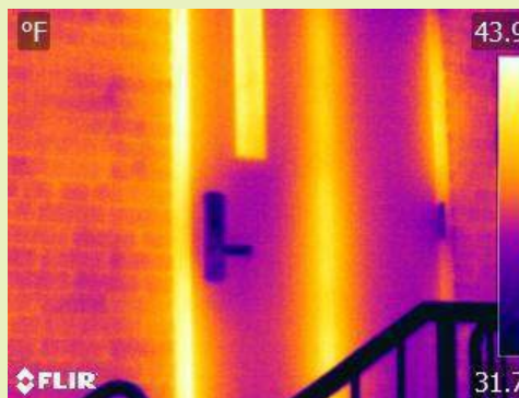
Bartlett Elementary Exterior Door Heat Loss
